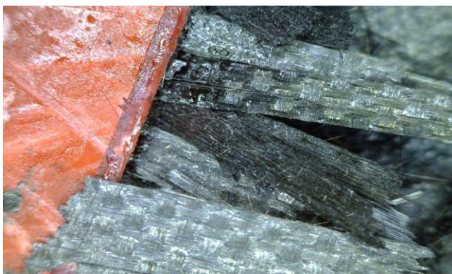
Fig. 13. Image of the fractured carbon fiber [2].
