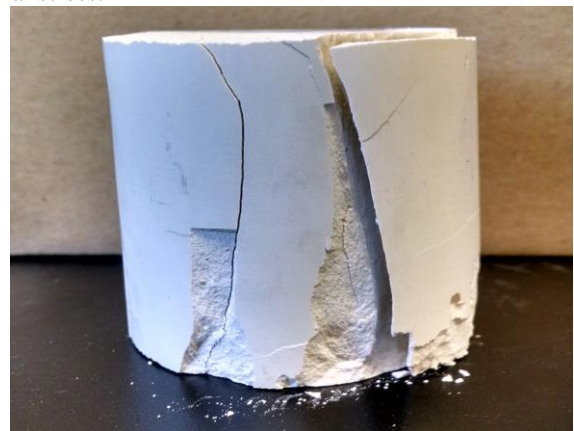
Fig. 15. Image of the Plaster of Paris experienced compressive loading [2].
